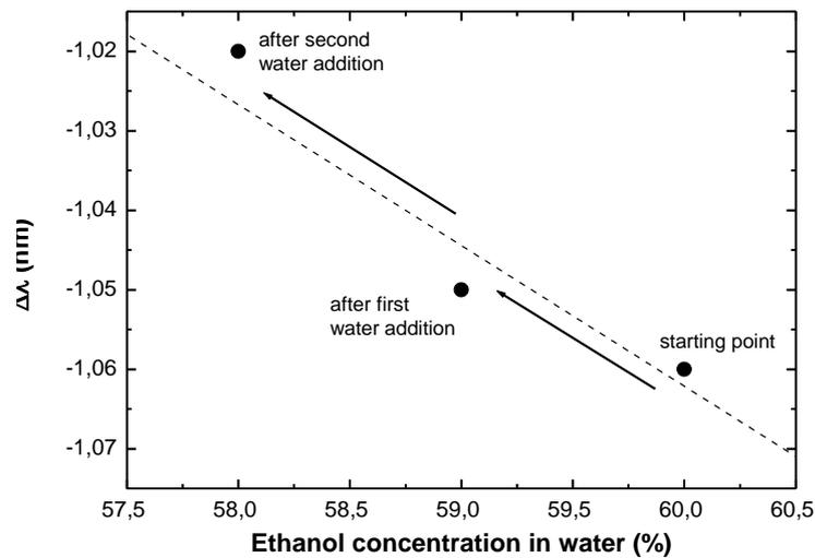
Fig. 7. LPG response when water is added to a sample with initial ethanol concentration of 60%, resulting in two consecutive decreases of 1% in the initial ethanol concentration. The dashed line corresponds to the best linear fit of figure 5.
