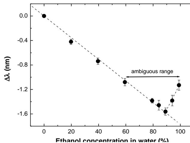
Fig. 5. LPG response measured in wavelength when immersed in samples of water with ethanol in different proportions and the best linear fit to samples with ethanol concentration lower and higher than 89.6%.
