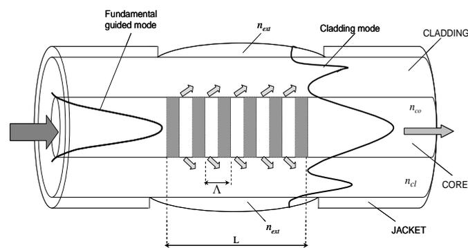
Fig. 1. LPG principle of operation.
