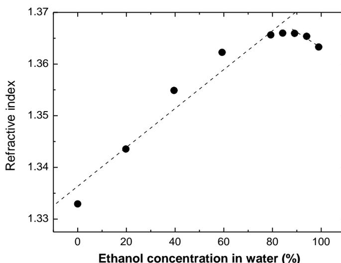
Fig. 3. Samples refractive indices measured with the Abbe refractometer and the best linear fit for samples with ethanol concentration lower and higher than 89.6%.
