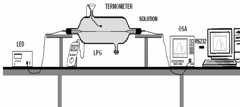
Fig. 2. Experimental set-up employed to characterize the LPG transducer.
