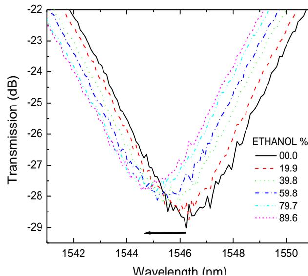
Fig. 4. Transmission spectra of LPG immersed in samples of water with ethanol in different proportions.
