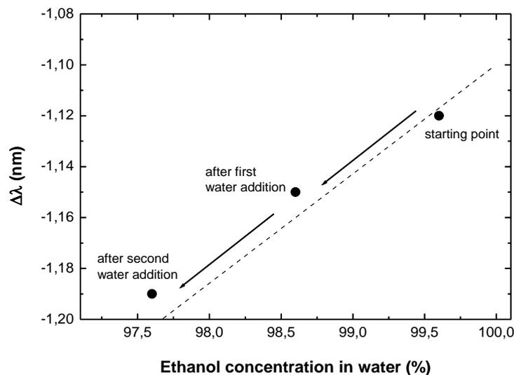
Fig. 8. LPG response when water is added to a sample with initial ethanol concentration of 99.6 %, resulting in two consecutive decreases of 1% in the initial ethanol concentration. The dashed line corresponds to the best linear fit of figure 5.
