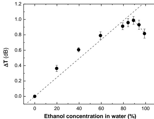
Fig. 6. LPG response measured in intensity when immersed in samples of water with ethanol in different proportions and the best linear fit to samples with ethanol concentration lower and higher than 89.6%.
