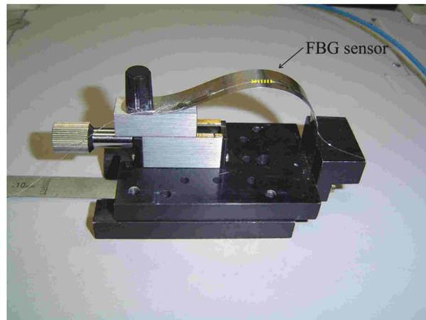
Fig. 1. FBG ( $\lambda = 1548.9$  nm,  $\Delta\lambda = 0.11$  nm at 21 °C) assembled in the sensing head.
