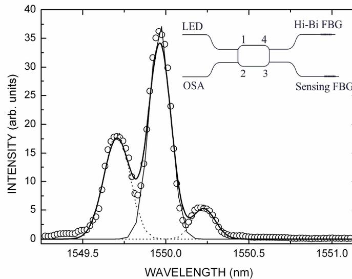
Fig. 4. Superimposed Hi-Bi and FBG sensing spectra obtained for a specific screw angle position. The experimental points (open circles) were adjusted by three Gaussians curves (HiBi-FBG: dotted, sensing: solid lines), and the bold solid line represents the resultant fitted curve.
