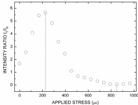
Fig. 7. Ratio of the intensities between the transmitted and reflected beams for several screw angle positions in the sensing head, obtained with the experimental setup of Fig. 2 and grating 2 (bandwidth of 0.15 nm and Bragg wavelength of 1549.24 nm at 21 °C).
