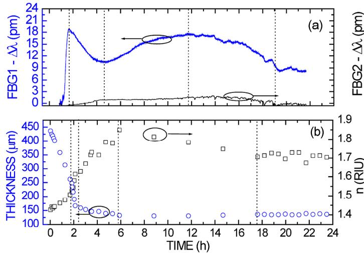
Figure 2. (a) Strain effects measured by FBG 1 and temperature changes indicated by FBG2, and (b) thickness and refractive index behavior measured with OCT throughout 24-hours drying process. Vertical dotted lines are used as a visual guide.
