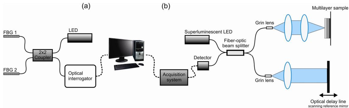
Figure 1. Heterogeneous sensor system: (a) FBG constituent and (b) OCT constituent.
