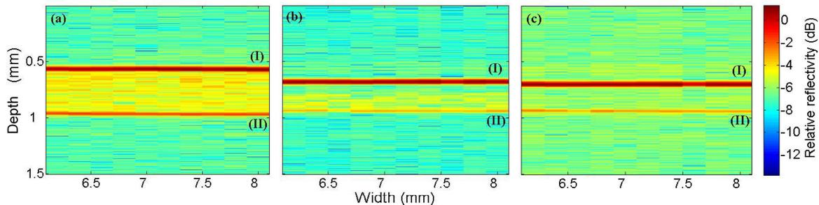
Figure 3. OCT images obtained at (a) 1.7, (b) 3.3 and (c) 10 hours. (I) air-film interface, (II) film-glass interface.
