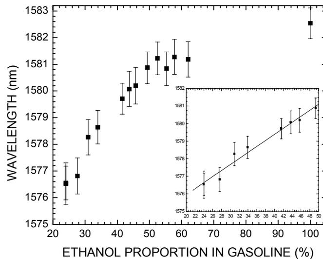
**Fig. 3. Peak position of the resonance band in the transmission spectrum of the LPG as a function of ethanol proportion (in volume) between 24 and 100 %. The insert shows the region with higher sensitivity (24 and 49 %), that can be described by a linear relation with angular coefficient of  $0.17 \pm 0.02$  nm/%.**
