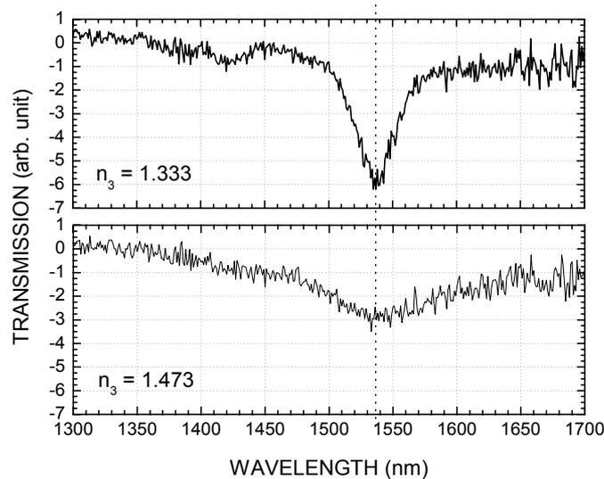
**Fig. 2. Transmission spectra of the same LPG comparing the attenuation dip for two different refractive indexes of the external medium: water (top) and a mixture of water and glycerine (bottom). The refractive index of the external medium is shown in the lower left corner of each graph.**
