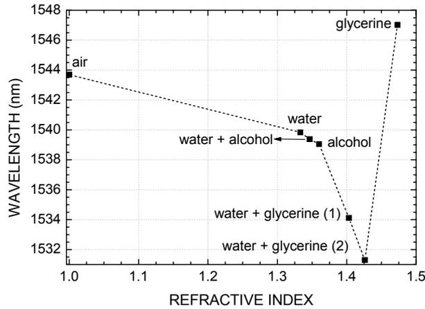
**Fig. 1. Peak position of the principal attenuation dip in the transmission spectrum of an LPG ( $\Lambda=649\ \mu\text{m}$ , 40 points) as a function of the refractive index of the external medium, in the range between 1.000 and 1.426.**
