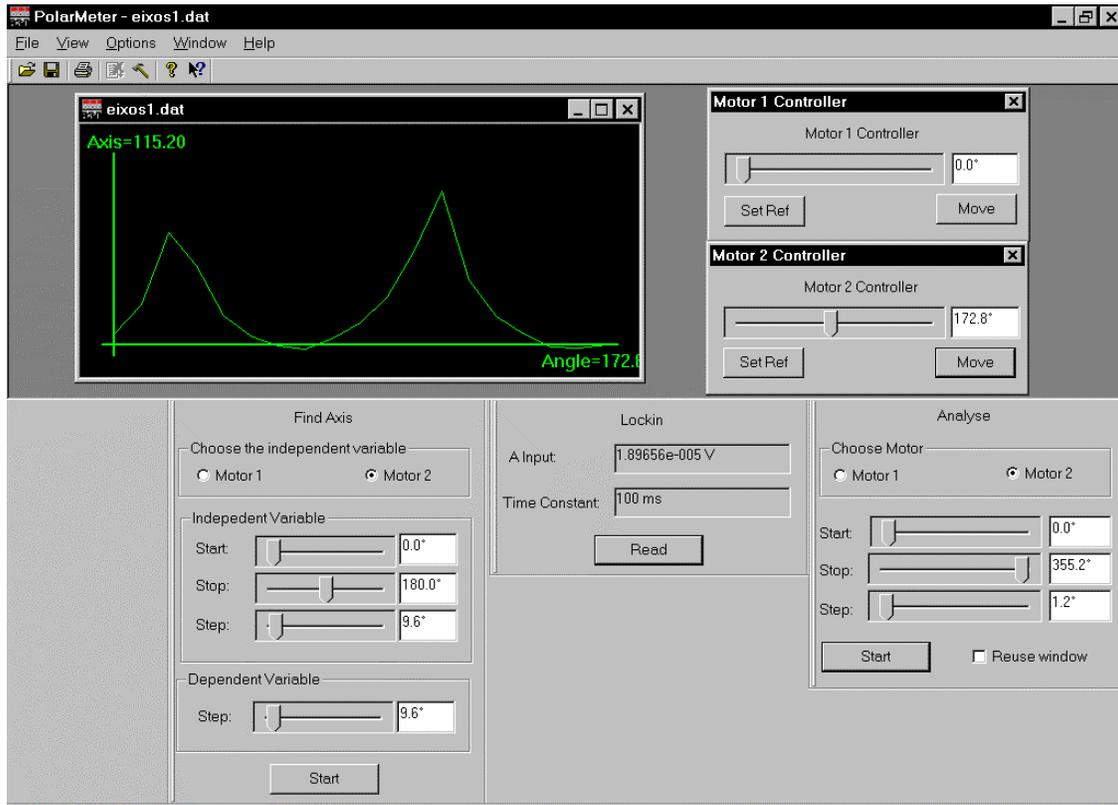
Figure 2: Aspect of the computer screen in the birefringence axis measurement.
