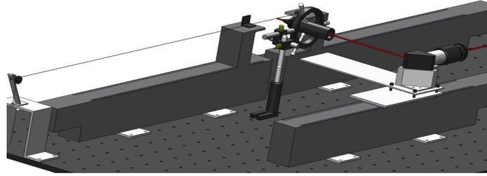
*Fig. 2 Configuration of the system to imprint LPGs. Beam from the CO<sub>2</sub> Laser in red, stages in gray; lens, beam expander and mirror in black, while fiber is depicted connected to a pulley and weight. Convergent lens is moved to the white aluminum platform when the machine operates as a taper rig and is set to produce a 3mm spot size on the fiber. When operating as an LPG imprinting system, the spot is set at 0.08–0.85mm.*
