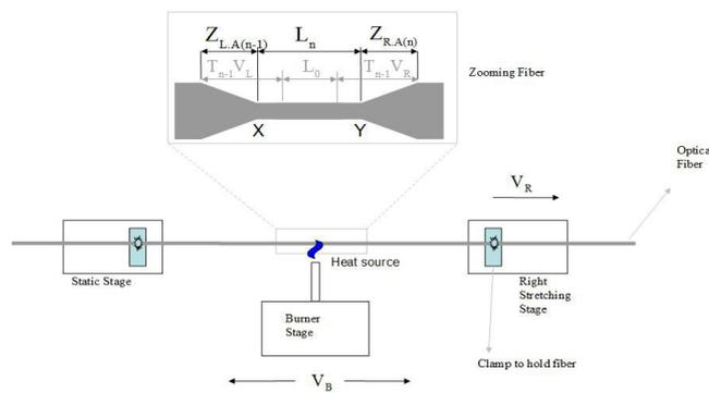
Fig. 1: Schematic description of the taper rig operating to produce a fiber taper with one static translation stage (left), a moving stretching stage to the right, a heat source stage heating a length  $L$  after the  $n$ -th sweep, and a zooming of the taper region depicting a step-taper with linear transition regions and a uniform waist between points X and Y.
