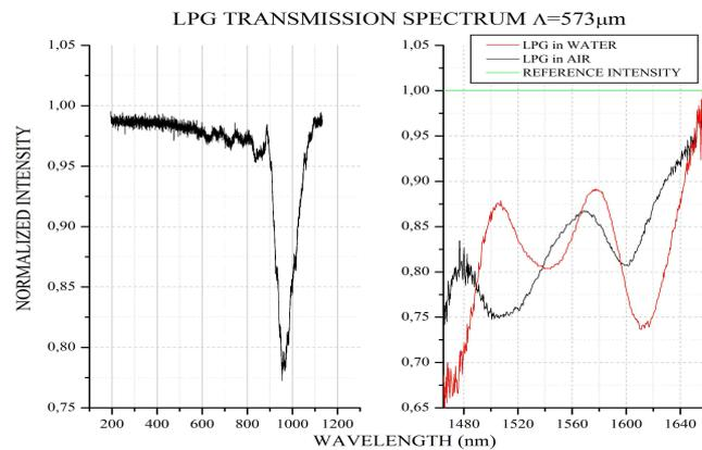
Fig. 3: Figure on the left side, the spectrum of the transmitted light in the near infrared range. In the figure on the right side, the spectrum of the transmitted light for an LPG immersed in air (black line) and in water (red line).
